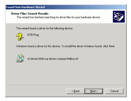
When USB bus driver ftdibus.inf is installed, Windows wants to install the virtual serial port driver, that makes the device to look like an ordinary COM port.
