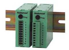
The I/O-transmitter 7180 is designed for serial transmission of alarm or switch information from or to the PC. Using this device you can eliminate internal I/O-cards for PC. This device also reduces the amount of wiring when connected with 2-wire RS-485 bus. Serial communication settings are made inside the case by selecting baud rate and the address of the device. Transmission of fast switching data is limited mainly by the baud rate and the application software.
