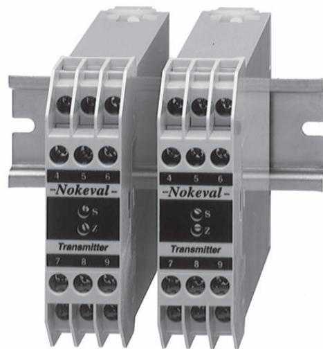
Signal converter 641 is designed to convert standard process input /output signals. Current inputs 0/4..20 mA can be converted into voltage outputs, -10..+10 V can be converted to 0..10 V, low mV inputs can be converted to standard outputs etc. Signal converter 641 accepts 2-wire transmitters without a separate power supply. Potentiometer input as a standard.
