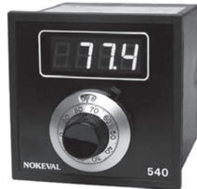
Setpoint controller 540 is designed for easy setpoint change. Output is adjusted via front panel 10-round potentiometer, setpoint can be locked up with mechanic friction lock. The setpoint potentiometer is selected to meet the demands of daily use. Display can be rescaled within limits -999..1999. The setpoint controller 540 is delivered according to an ordered range and output, standard display range is 0-100.0 and output 4-20 mA. Display and output range can be changed later inside of case.
