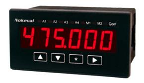
The panelmeter 2071 is designed for serial communication. It uses the simple Nokeval SCL protocol where only the address, value and check sum are sent. The panelmeter has both the serial inputs RS-232 and RS-485 as a standard. The serial bus is galvanically isolated from the processor and the power supply. In the configuration mode you can set the address, baud rate and the type of number value that you want to appear on the display after power connection.
