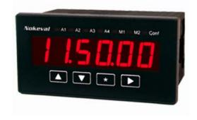
The panelmeter **2066** is designed for industrial timing. A typical application is heat treatment in metal industry. The timing starts when the furnace door is closed or the required temperature is reached.
