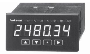
The panelmeter 2028 is specially designed to satisfy the needs of massflow indication in difficult applications where other flowmeters are unsuitable or difficult to use, such as measurement of solid matters or molten metal. Based on the current signal of a strain gauge transmitter the panelmeter 2028 calculates the change of the weight per second and in that way shows the actual flow rate.
