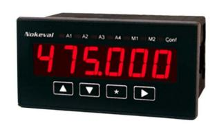
The panelmeter 2026 is designed for analog signals in cumulative counting applications. The display indicates flow volume per a time unit and it can be freely scaled in the desired engineering units via front panel keys.
