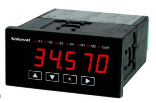
The panelmeter 2011 is designed for usual process inputs 0/4..20 mA, 0..5/10 V and for potentiometers 100 ohm.. 10 kohm. Selection of the sensor type and display scaling is easy via front panel keys. 2 alarm relays with change-over contacts are available as an option. Alarm limits and hysteresis are freely selectable via front panel keys. The display can be damped by a digital filter if necessary. The number of decimals is selectable. The brightness of the display can be selected as well.
