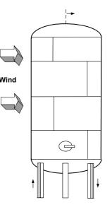
In tank applications the wind decrease accuracy when sensors are connected in parallel. The serial connection of signals gives exact sum of sensors in all loading conditions.
