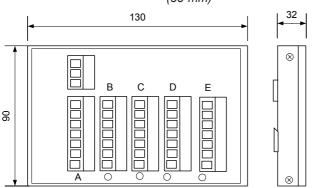
Each sensor is connected separately to terminal block (B-E) using 6 wires. Panelmeter is connected to terminal block A. In case that all 4 bridges are not used, terminals 3 and 4 must be shortcircuited in unused terminal blocks.
