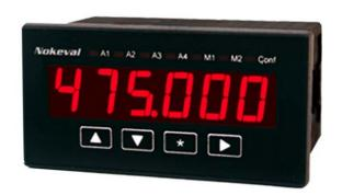
The panelmeter 2064 is designed to display the position of incremental sensors. The incremental sensor has two output channels and the direction of rotation is indicated on the basis of the phase shift of the channels A and B. The panelmeter counts the number of pulses from both the sensor outputs and the channel whose pulse edge rises up first determines the direction of rotation.
